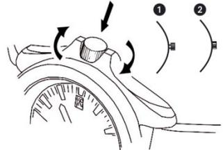
**IMPORTANT:** After every time you change the time or date, make sure that the crown is screwed back in to ensure that the watch remains watertight. Under no circumstances should you ever use force or tools to unscrew the crown or screw it back in place!
