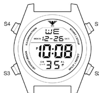
Push button S3 once to change from one display mode to another. In any setting mode, if there is no key manipulation for approximately 1-2 minutes, the watch will automatically save the entered data and exit the setting mode.
